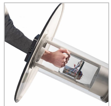
The electronics can be serviced without using any tools thanks to a removable gear tray.
