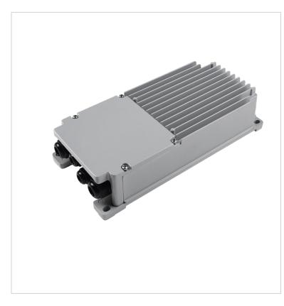
Class I non-insulated, 600W output constant current DALI-2 programmable. An IP66 enclosure makes it also suitable for outdoor applications and its electrical characteristics make it suitable for TV broadcasting applications.
